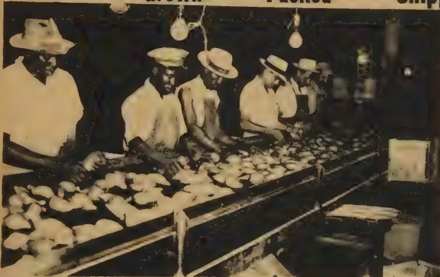
The above Yams have been washed and are in the grading process. The U. S. No. 2's are being graded out and the U. S. No. 1's are continuing on the conveyor into the waxing machine.
