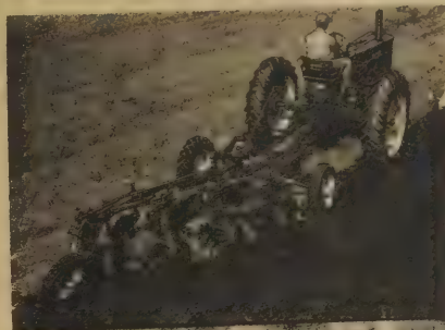
Today's John Deere leaders are truss-frame plows, a full line designed throughout for greater strength and clearance. These husky plows are available both in tractor-drawn types and for "pick up and go" fully integral operation.
