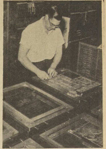
After the reporter writes his story, it is set in metal type on a linotype machine and placed into chases in the newspaper composing room.
